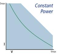
Constant power mode simulates a load whose power consumption is independent of the applied voltage.
