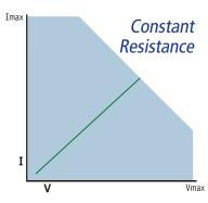
Constant resistance mode simulates a standard resistive load by providing a current drain proportional to voltage. Settings are displayed in Ohms or milli-Ohms.
