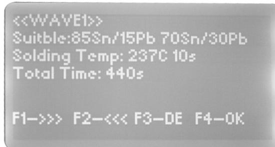
When selections are complete, then Press "F4" button to return previous page. Press the temperature wave that the "F1" key carries out to make selection automatically. When it is ending, the work will shut down automatically, and the warning buzzer is working.
